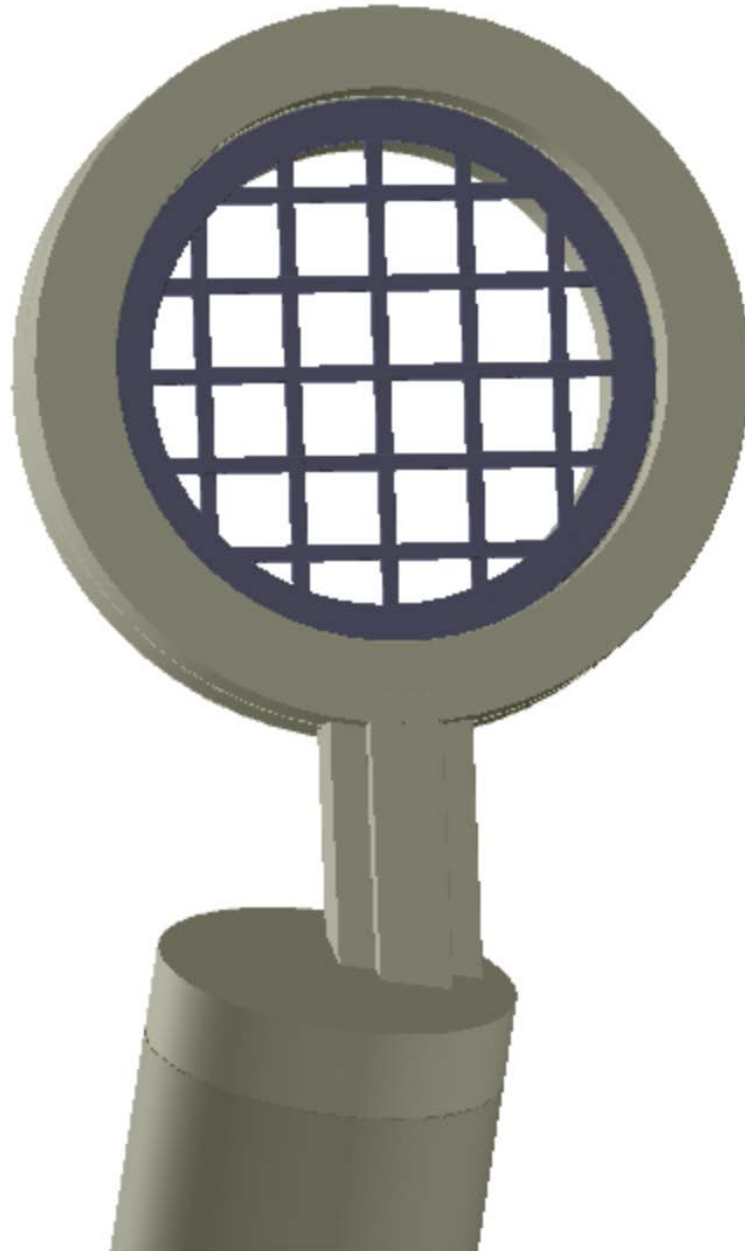
Figure 4.9: VisRad illustration of the configuration used for experimental calibration. A copper mesh target was used to determine the resolution of the radiography setup. The mesh strips are 0.08 mm wide and 0.02 mm thick.
