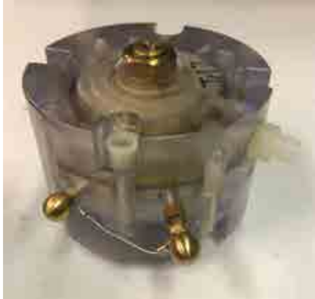
Figure C.3: An L3Harris spark-gap switch with brass electrodes, capable of operation at 200 kV ( \pm 100 kV) and up to 200 psi gas fill. These switches are used in the MAIZE and BLUE LTD systems at the University of Michigan. In this image, the switch is shown with a shorting wire between the UV-pin and mid-plane. In the BLUE cavity, the shorting wires are replaced with 3 m \Omega resistor chains for proper operation of the UV-pin.
