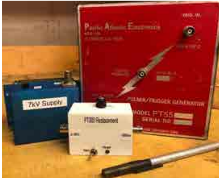
Figure C.7: The Pacific Atlantic Electronics PT55 module with a +7 kVDC power supply and the newly developed +300 V pulse generator (PT003 replacement). Together, these modules can produce a +50 kV output pulse with <10 ns jitter from a logic-level (+5 V) input pulse.
