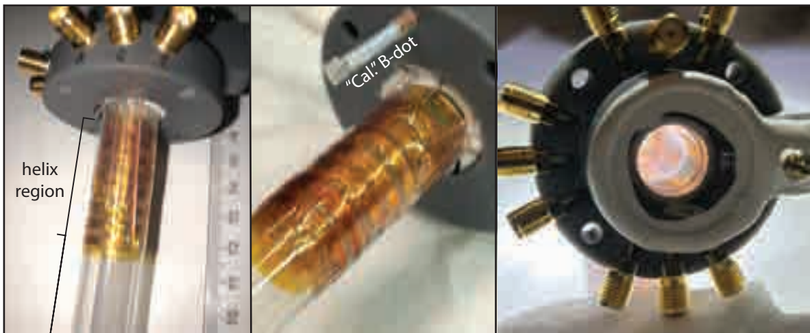
Figure 3.37: Newer excluded flux B-dot probe design using crescent-shaped loops covering 1/4 the circumference of the discharge tube. Photographs on the bottom show eight of the flux loops installed on a discharge tube, as well as the calibration B-dot that is sensitive to azimuthal flux in the return current structure outside the helix (essentially measuring current in the helix).
