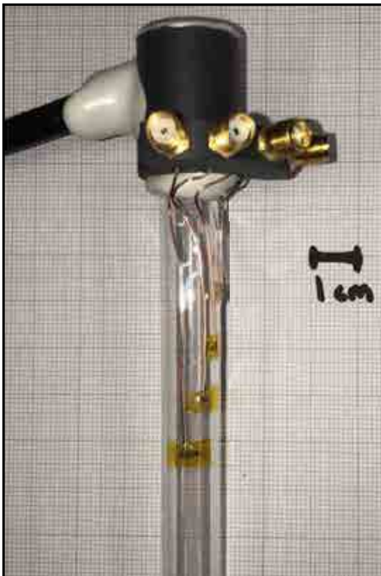
Figure 3.33: Early “B-dot discharge tube” with four external micro B-dots for measuring B_e at various axial heights on the top half the discharge tube. The B-dots on this tube were insulated with clear, high dielectric strength heat-shrink tubing approximately 0.5 mm in thickness.
