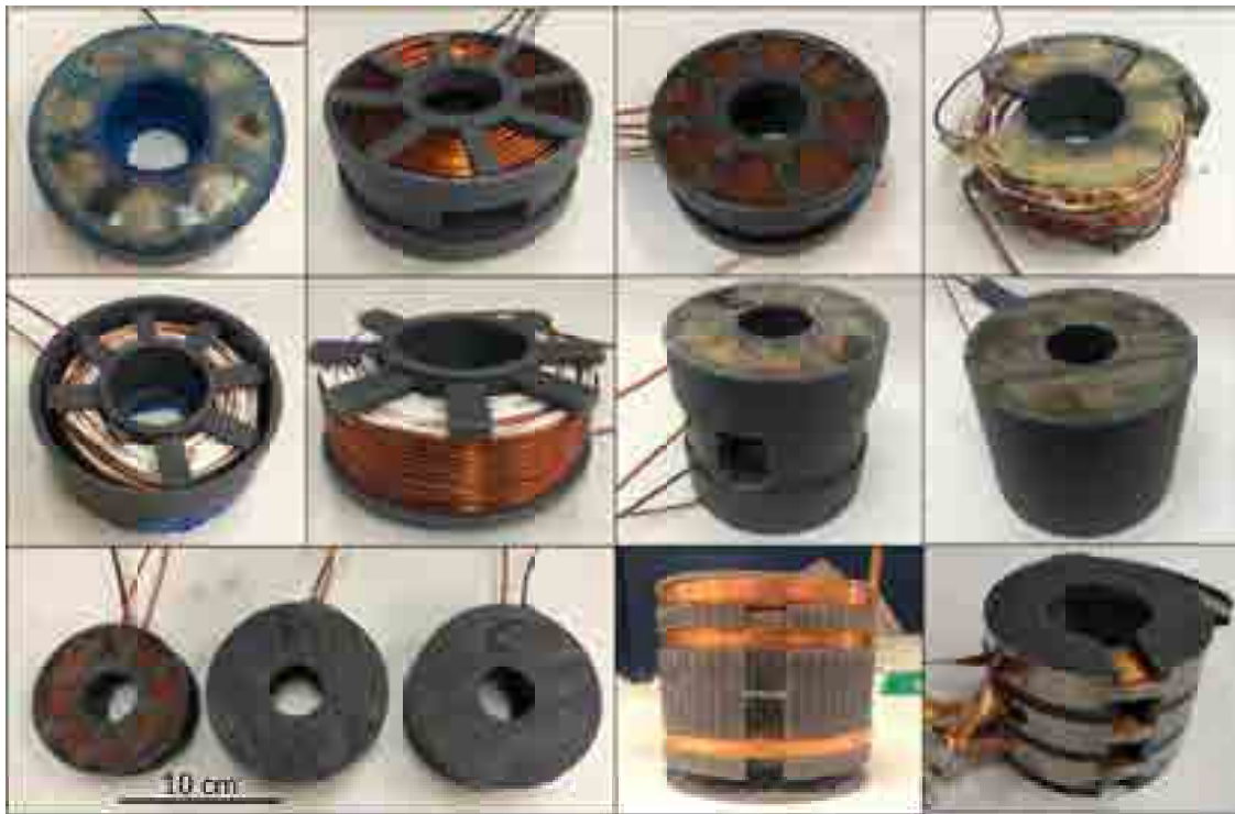
Figure 3.7: An assortment of bias coils made in-house for FRC experiments on MAIZE. Coils were made by manual winding of enameled wire or copper strip on 3D printed resin frames and potted in flexibilized Epon 8131. Peak (non-destructive) fields reached with later coils were around 3–4T.
