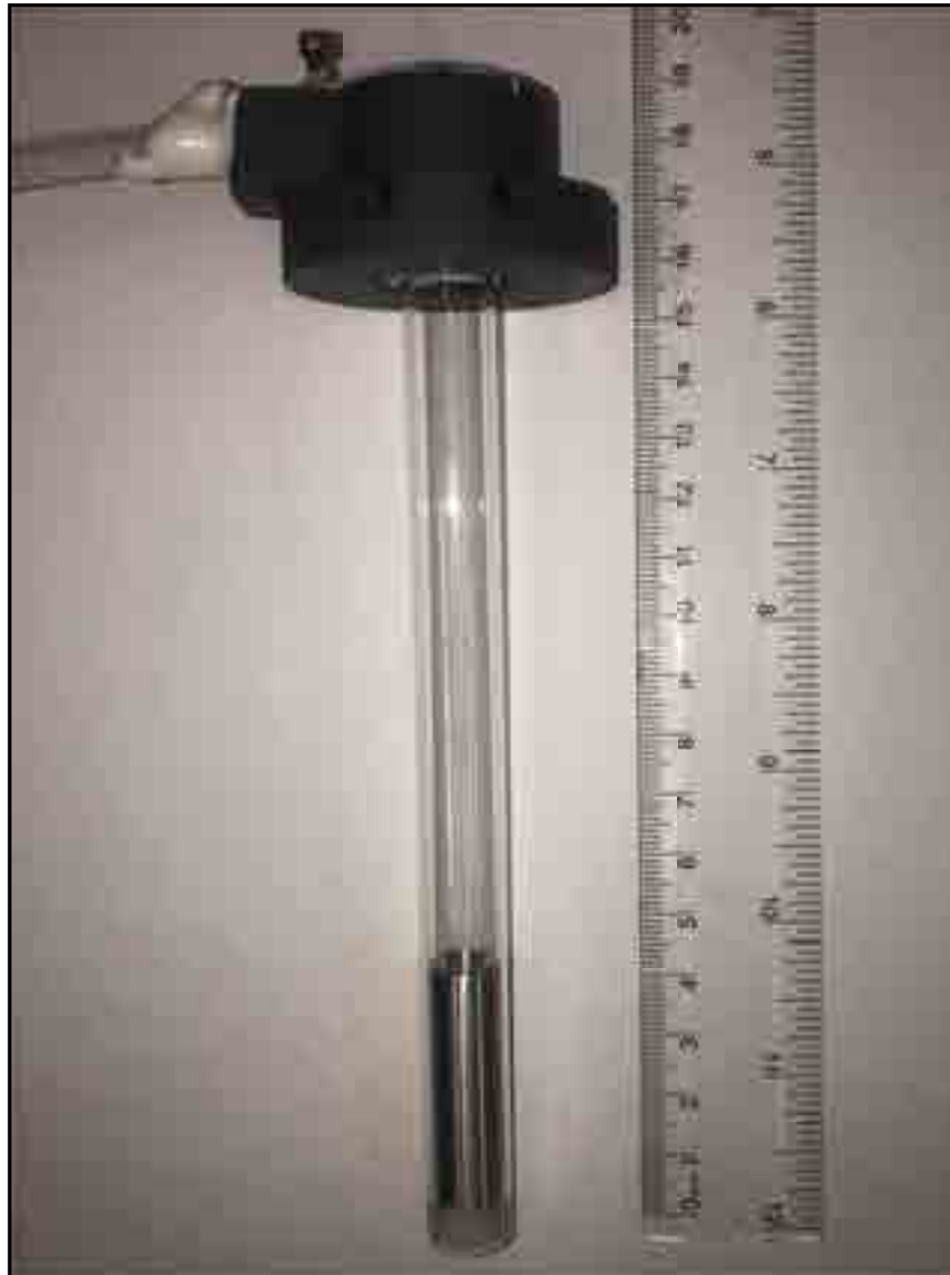
Figure 3.4: A later generation of discharge tube used in the “final” hardware of Section 3.10. Top ZPI ring is not visible. Hexagonal holes in the top (plastic) manifold are for SMA connectors of micro B-dots, which are not installed on this tube (see Section 3.13).
