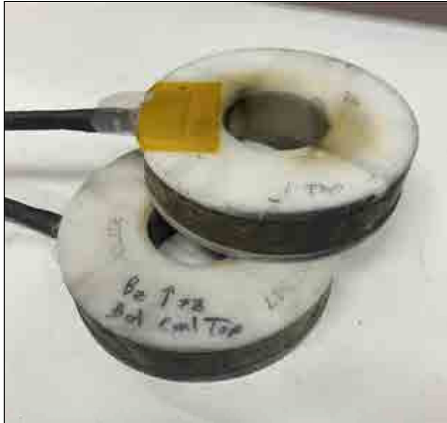
Figure 3.8: A pair of 2" (5 cm) ID coils made at SNL for applied bias fields on the Z-machine. With the limits of the capacitor bank at PPML, the pictured coils can produce a peak on-axis field of 5–6 T depending on their spacing. These coils were used in FRC experiments on MAIZE, as shown in Fig. 3.22.
