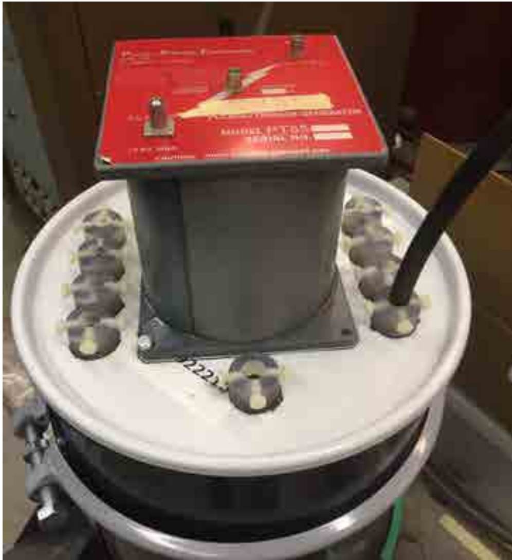
Figure C.6: The 10-gallon oil drum containing the trigger pulse generating brick, which is charged in parallel with the BLUE LTD cavities and triggered by the PT55 pulse generator mounted to the top of the drum.
