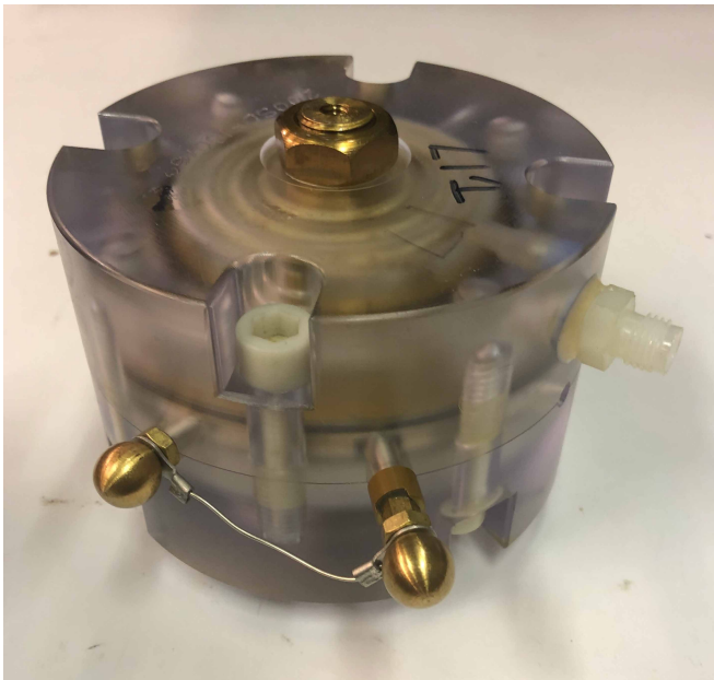
FIG. 3. An L3Harris spark-gap switch with brass electrodes, capable of operation at 200 kV ( \pm 100 kV) and up to 200 psi gas fill. These switches are used in the MAIZE and BLUE LTD systems at the University of Michigan. In this image, the switch is shown with a shorting wire between the UV-pin and mid-plane. In the BLUE cavity, the shorting wires are replaced with 3-M \Omega resistor chains for proper operation of the UV-pin.
