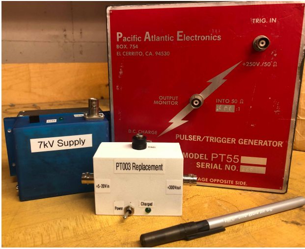
FIG. 7. The Pacific Atlantic Electronics PT55 module with a +7 kVDC power supply and the newly developed +300 V pulse generator (PT003 replacement). Together, these modules can produce a +50 kV output pulse with <10-ns jitter from a logic-level (+5 V) input pulse.
