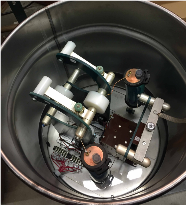
FIG. 5. A 20-gallon oil drum contains the three Ross HV relays used in the charging circuit. The relays are operated by the control panel (see Sec. III A and Fig. 4) during the charging sequence. The large copper-sulfate dump resistors in this photograph were ultimately replaced with 50-k \Omega ceramic resistors.
