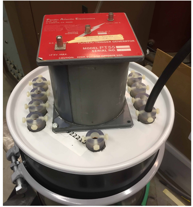
FIG. 6. The 10-gallon oil drum containing the trigger pulse generating brick, which is charged in parallel with the BLUE LTD cavities and triggered by the PT55 pulse generator mounted to the top of the drum.
