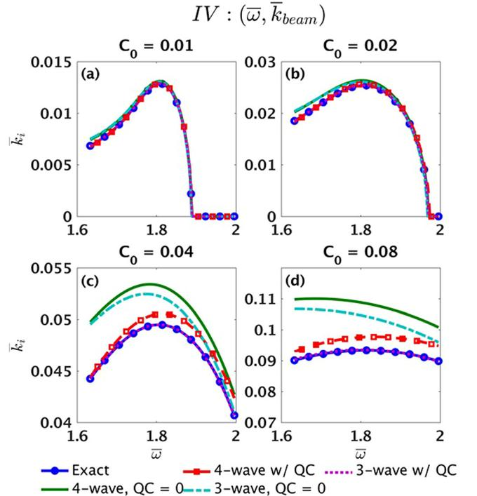
FIG. 6. The value of  $\bar{k}_i$  as a function of  $\bar{\omega}$  from the exact theory and from Pierce's 3-wave and 4-wave theory using approximation IV applied to  $Q_3$ , for (a)  $C_0 = 0.01$ , (b)  $C_0 = 0.02$ , (c)  $C_0 = 0.04$ , and (d)  $C_0 = 0.08$ . In each graph, Pierce's theory with and without the effect of  $Q_3$  is shown.
