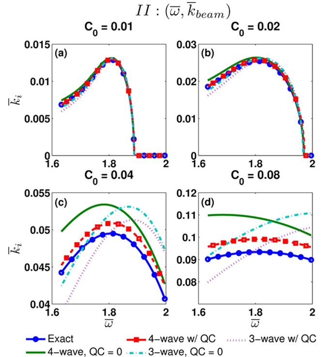
FIG. 4. The value of  $\bar{k}_i$  as a function of  $\bar{\omega}$  from the exact theory and from Pierce's 3-wave and 4-wave theory using approximation II (Eq. (13b)), for (a)  $C_0 = 0.01$ , (b)  $C_0 = 0.02$ , (c)  $C_0 = 0.04$ , and (d)  $C_0 = 0.08$ . In each graph, Pierce's theory with and without the effect of Q is shown.
