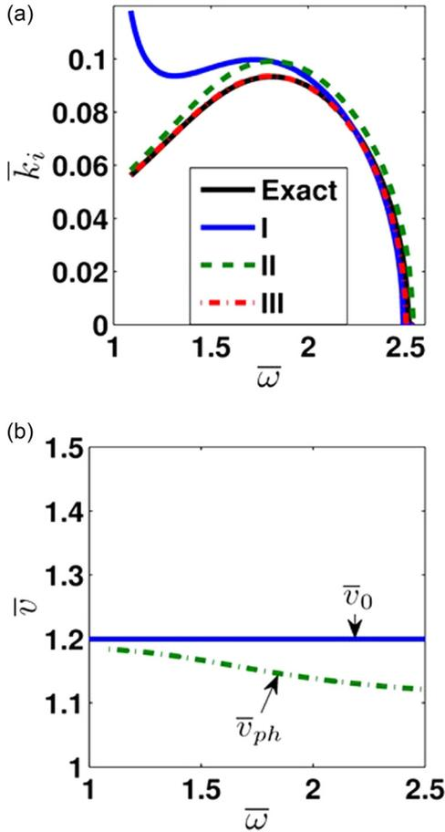
FIG. 2. (a) Top: The value of  $\bar{k}_i$  as a function of  $\bar{\omega}$  for  $C_0 = 0.08$  according to the exact theory and to Pierce's 4-wave theory [Eq. (6)] using approximations I, II, and III. (b) Bottom: The plot of normalized phase velocity,  $\bar{v}_{ph} = \bar{\omega}/\bar{k}_r = \omega/k_r c_e$ , for the amplifying wave, and the normalized beam velocity  $\bar{v}_0 = v_0/c_e$ .
