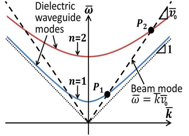
FIG. 1. The normalized dispersion diagram for the first two waveguide modes ( $n = 1$  and  $n = 2$ ) and the beam mode in a dielectric TWT, with possible operating points at  $P_1$  and  $P_2$ . This paper considers operation at  $P_1$  and is normalized accordingly:  $\bar{\omega} = \omega/\omega_{c1}$ ,  $\bar{k} = kc_\epsilon/\omega_{c1}$ , and  $\bar{v}_0 = v_0/c_\epsilon (>1)$ . The cutoff frequency is at  $\bar{\omega} = 1$ , and the slope of the dielectric light line is unity.
