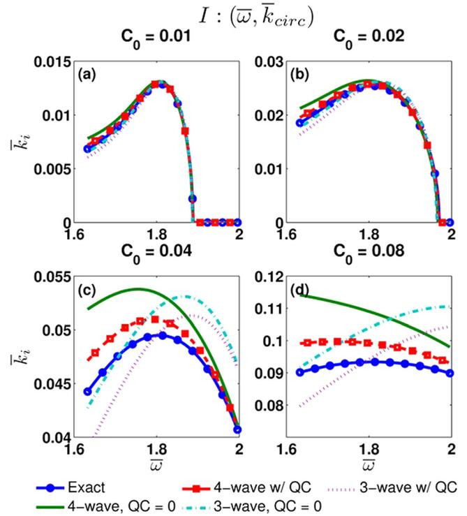
FIG. 3. The value of  $\bar{k}_i$  as a function of  $\bar{\omega}$  from the exact theory and from Pierce's 3-wave and 4-wave theory using approximation I (Eq. (13a)), for (a)  $C_0 = 0.01$ , (b)  $C_0 = 0.02$ , (c)  $C_0 = 0.04$ , and (d)  $C_0 = 0.08$ . In each graph, Pierce's theory with and without the effect of Q is shown.
