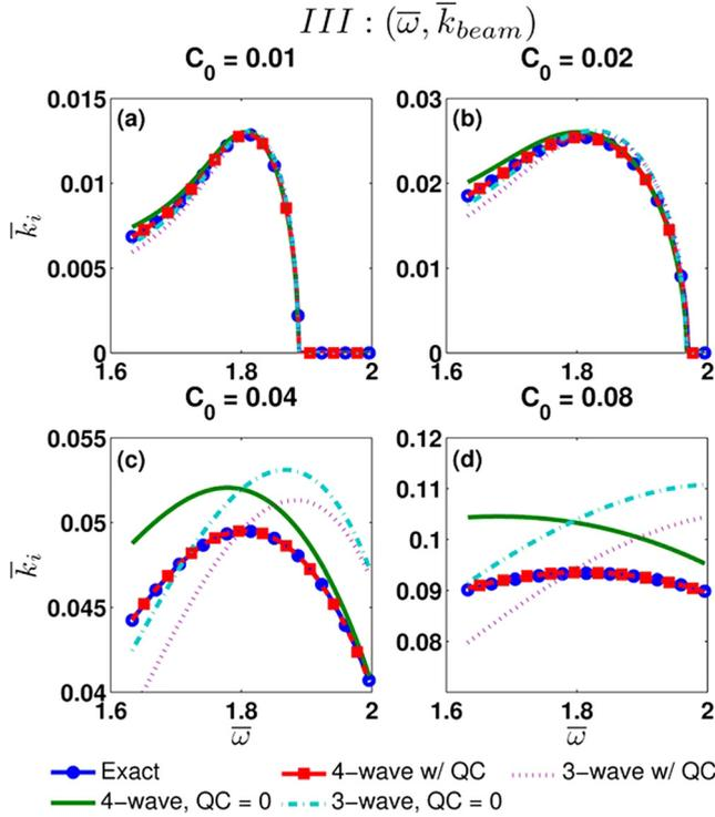
FIG. 5. The value of  $\bar{k}_i$  as a function of  $\bar{\omega}$  from the exact theory and from Pierce's 3-wave and 4-wave theory using approximation III (Eq. (13c)), for (a)  $C_0 = 0.01$ , (b)  $C_0 = 0.02$ , (c)  $C_0 = 0.04$ , and (d)  $C_0 = 0.08$ . In each graph, Pierce's theory with and without the effect of Q is shown.
