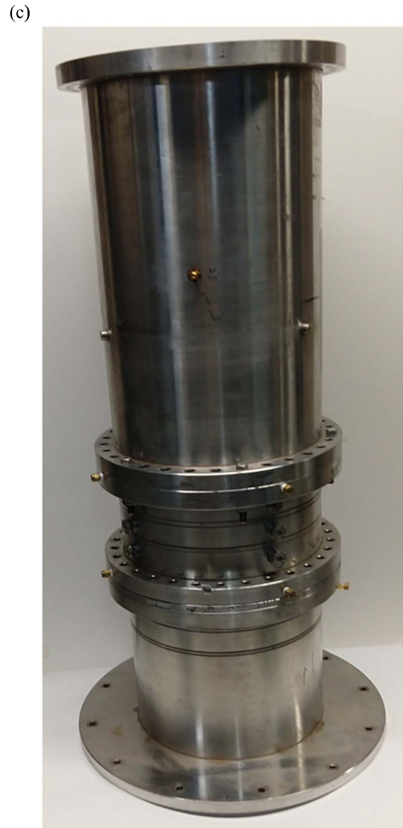
Fig. 8. (Continued.) (c) Brazed GW-class MILO to be tested experimentally on the BLUE LTD facility.
