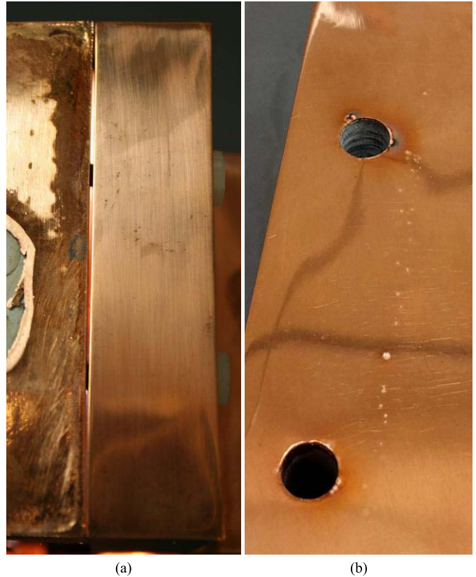
Fig. 7. Uneven electroplating leading to (a) poor electrical contact at unions and (b) arcing between the parts during operation.
