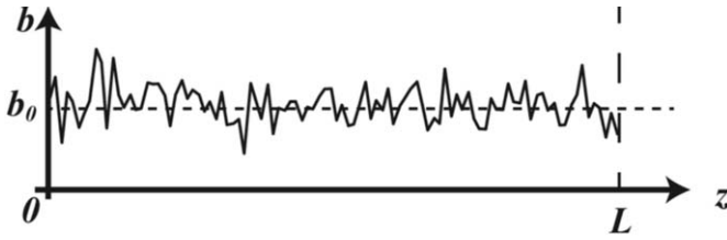
Fig. 1. Example of random variations along the tube axis; b is Pierce's detune parameter.
