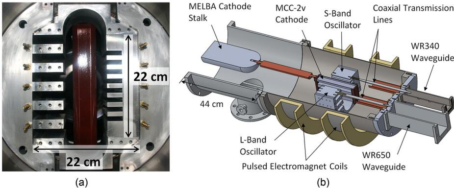
FIG. 1. Experimental hardware and configuration. (a) Photograph of MFRPM prototype viewed from the front. The central structure is the cathode. The anode consists of 6-cavity 1 GHz and 8-cavity 2 GHz planar cavity arrays. (b) Cross-sectional view of the experimental configuration.
