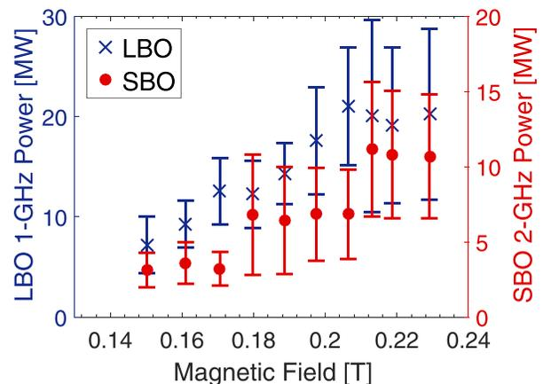
FIG. 3. Experimental powers for both oscillators vs. magnetic field.
