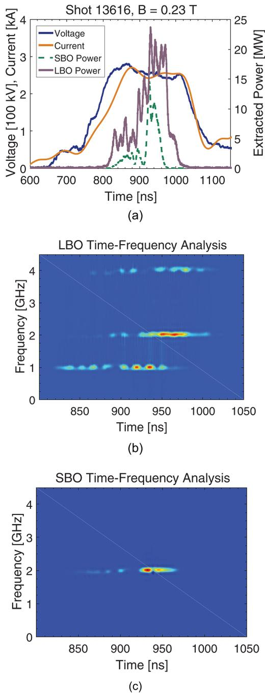
FIG. 2. Sample experimental MELBA-C shot no. 13616. (a) Shot plot illustrating voltage, current, and detected RF powers for both oscillators. Peak LBO (SBO) powers were 24 MW (15 MW) at 0.98 GHz (2.0 GHz). (b) Time-frequency analysis for the LBO. (c) Time-frequency analysis for the SBO.
